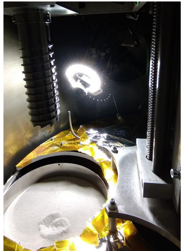
Figure 26: Image of the VSVA++ inside the LUVMI-X thermal vacuum test setup at TUM
